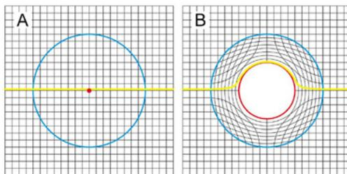
**Figure 9:** *Principle of cloaking. a) A simple square grid. b) After applying an appropriate coordinate transformation, a distorted square grid with a hole in the middle is obtained. Used from (Leonhardt 2011).*
