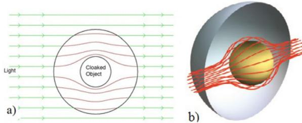
**Figure 5:** a) Two dimensional cross section of the cloaking system showing the direction of rays inside and outside the metamaterial. Rays are diverted away from the cloaked circular area and emerge undisturbed from their original course, just as if it propagated through free space. Used from (Dodson 2013).
