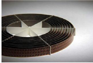
**Figure 6:** *The structure of the two dimensional cylindrical cloaking structure. The shape of SRRs varies gradually in the structure at every cylinder. Used from (Gbur 2011).*
