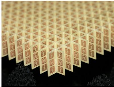
**Figure 4:** *Components of a negative refractive index metamaterial. These consist of copper SRRs and copper wire strips on a fibre glass circuit board material assembled in an interlocking lattice. Each unit cell has dimension of 5mm. Used from (Johnson 2008).*
