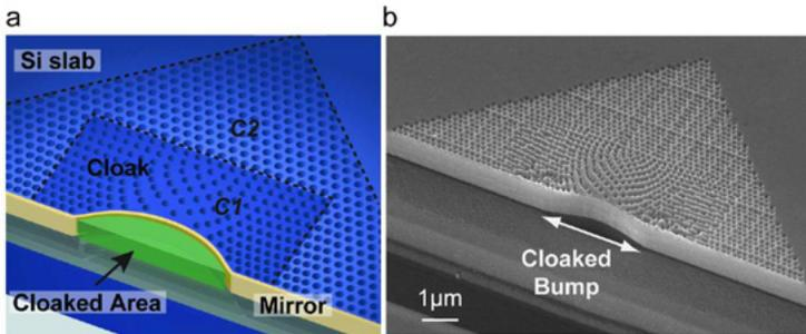
**Figure 8:** *a) Diagram of the structure of the carpet cloak. The triangular region (C2) has a uniform hole pattern and serves as a background medium with constant effective refractive index. The rectangular region C1 has a variable index profile. b) SEM image of the structure of the carpet cloak. Used from (Yaris 2009).*
