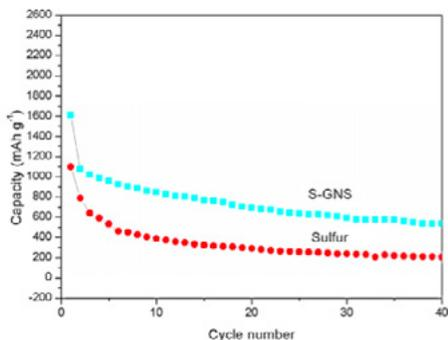
*Figure 3: Capacity of pure sulfur, S-GNS battery systems vs. cycle number. It can be observed that the S-GNS composite had a higher initial capacity than the pure sulphur, and maintained better cycling stability. (Wang, J. Z. et al 2010)*
