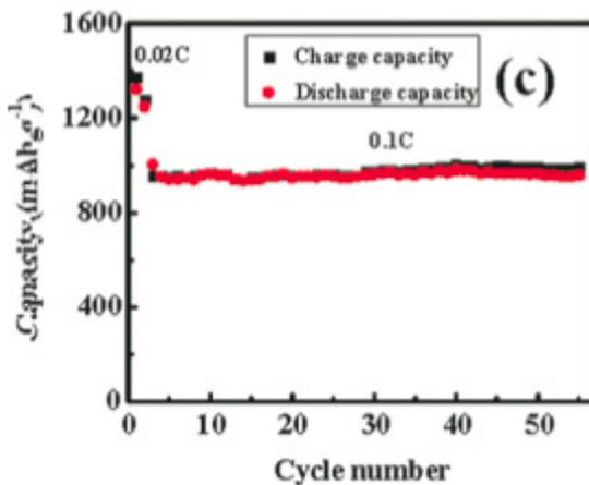
Figure 6: Graph depicting the cycle performance at constant rate of 0.1 C. Can be seen that the capacity remains near initial levels, even during the final cycles (Ji, L. et al 2011).
