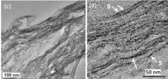
**Figure 4:** TEM images of Nafion-coated FGSS nanocomposite, at scales of 100nm (c) and 50nm (d). The sandwich structure of interlocking dark (sulphur) and bright (graphene) lines can clearly be seen (Cao, y. et al 2011).
