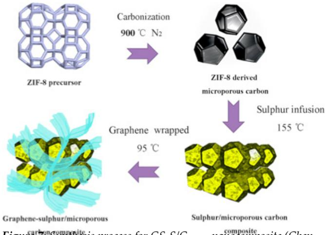
**Figure 7:** Synthesis process for GS-S/ $C_{ZIF8-D}$  nanocomposite (Chen, R. *et al.*, 2014)
