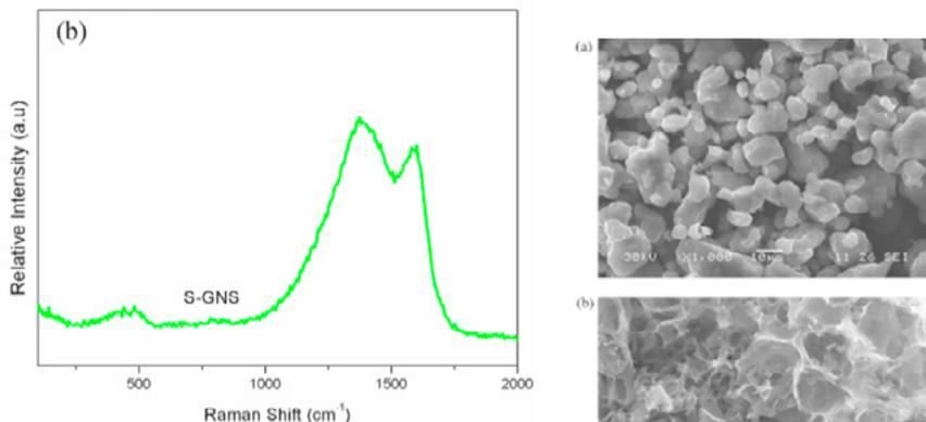
**Figure 1:** Raman Spectrum of S-GNS composite. No characteristic peak for sulfur was observed (normally found at 259, 412  $\text{cm}^{-1}$  (White, S. N., 2008)), indicating that the sulfur was in a highly dispersed state throughout the composite (Wang, J. Z. et al 2010).
