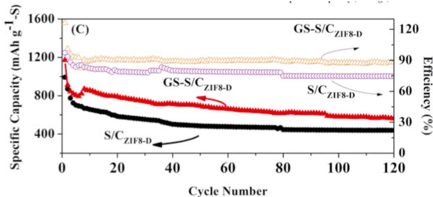
**Figure** Cycling performance of GS-  $S/C_{ZIF8-D}$  composite compared to the  $S/C_{ZIF8-D}$  composite. Can be observed that the capacity retention is significantly improved for the GS-  $S/C_{ZIF8-D}$  composite compared to the  $S/C_{ZIF8-D}$ . (Chen, R. *et al* 2014).
