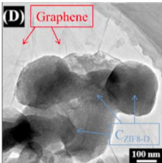
**Figure 8:** SEM image of graphene-wrapped MOF derived microporous carbon framework. Due to the flexibility of graphene, it can easily wrap around the GS-S/ $C_{ZIF8-D}$  nanocomposite. (Chen, R. *et al.*, 2014)
